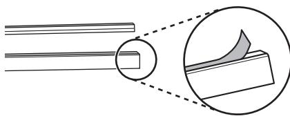
5 Attach the black coloured lower strip ① to the bottom of the lower cover.
