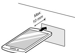
**3** Press and hold the **Download Cycle** button for 3 seconds or longer while holding the smartphone mouthpiece to the logo until the data transfer is complete.
