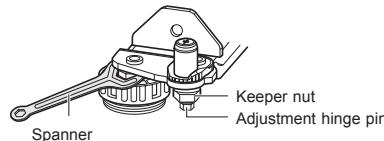
1 Loosen the keeper nut by rotating it counterclockwise using a 19 mm spanner.
