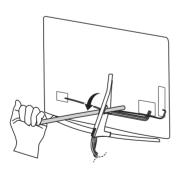
Do not use a sharp object when you detached the cable cover. This could damage the cable or the cabinet. It may also cause personal harm. (Depending on model)
